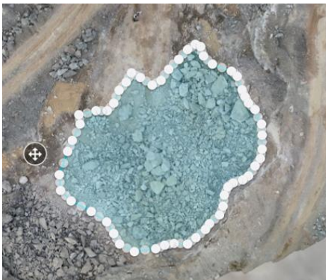
Figure 11: Demarcating the Blast Area
