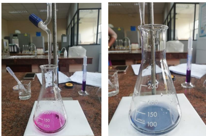
Figure 3.2: Color changes observed during the Calcium and Magnesium test
